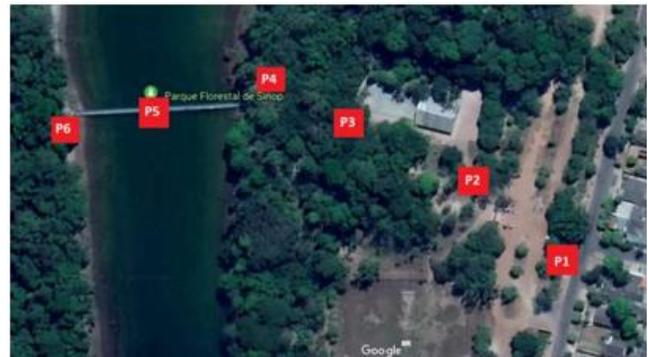
**Figure 6:** Positioning of acoustic measurement points in the Parque Florestal.
