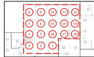
**Figure 1:** Boundaries of measurement test area. Circles identify 18 loudspeakers, as well as measurement locations. The three-LSCZ are 1-2-3, 4-5-16, 7-8-9, 10-11-12, 6-14-15 and 13-18-17. The six-LSCZ are 1-2-3-4-5-16, 6-7-8-9-10-15 and 11-12-13-14-17-18.
