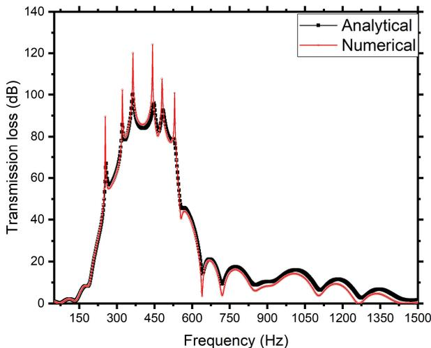
**Figure 2:** Comparison of theoretical and numerical Transmission loss.
