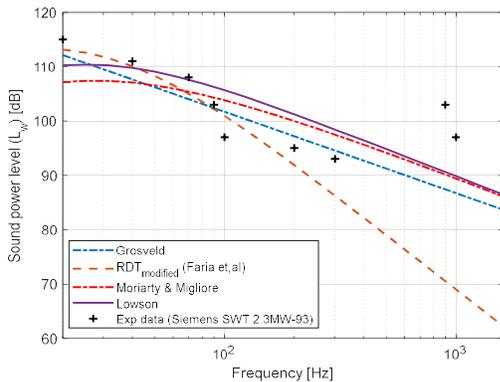
**Figure 1:** Comparison of the turbulent inflow noise predicted from the Grosveld, Moriarty, Lawson, and modified RDT models at mean wind speed of 12 m/s, at turbulence intensity of 10%, and validated with experiment data of Siemens SWT 2.3 MW-93 model.
