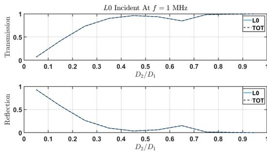
**Figure 4:** Energy transmission and reflection for the incidence of an L0 propagating mode at a frequency of 1 MHz as a function of the diameter ratio  $D_2/D_1$  between the reducer and the base waveguide.
