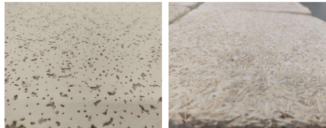
a) Conventional mineral fiber-based acoustic ceiling tile
