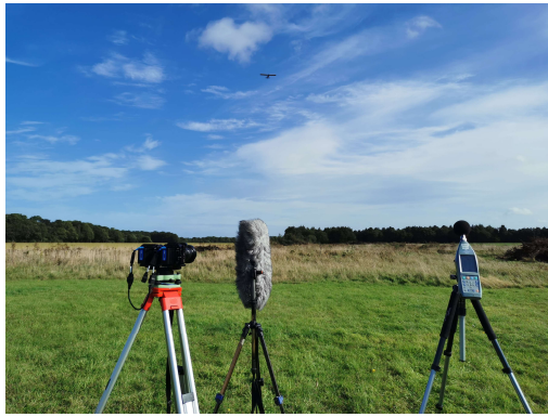
Figure 2: Measurement set-up to capture aircraft flyover - from left to right: video camera, ambisonic microphone, sound level meter.
