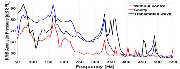
**Figure 4:** Experimental pressure level in the cavity
