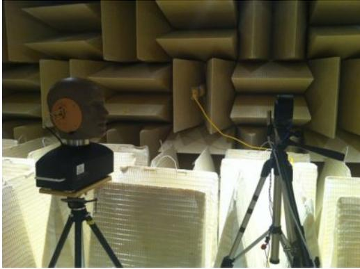
Figure 3: Test set-up in the anechoic room
