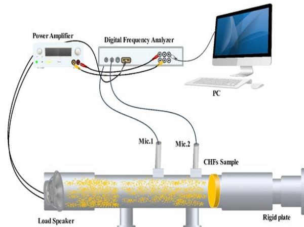
Figure 2: Impedance tube schematic.
