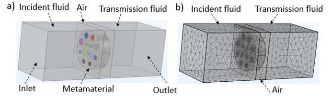
**Figure 2:** Periodic unit cell for TL evaluation (a) geometry of the PUC (b) mesh of the PUC.
