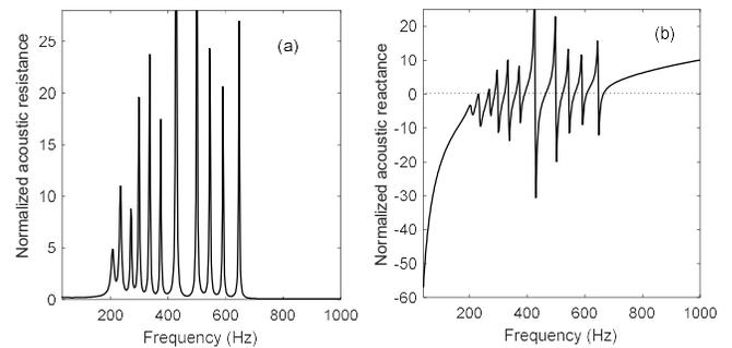
Figure 4: Normalized surface impedance of the metamaterial (a) acoustic resistance (b) acoustic reactance.
