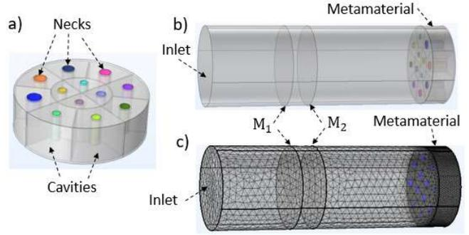
**Figure 1:** Numerical models (a) metamaterial based on twelve parallel resonators (b) geometry (c) mesh.
