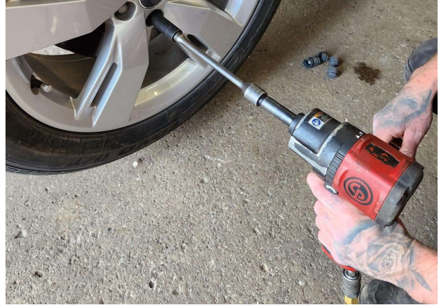
Figure 1. Air impact wrench tightening a wheel bolt
