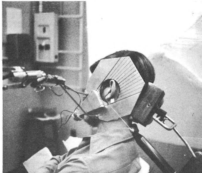
Fig. 4. Measurement of blocked-meatus response using a probe microphone (lower right) and a special source designed to generate well-defined progressive waves at grazing incidence. From SHAW (1974a, 1975).
