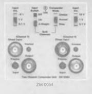
Two Channel Compander ZM 0054 for automatic level regulation with two of the FM, Direct or Vibration Units. Facilitates unattended recording and enables non stationary signals with dynamic range of over 70 dB to be recorded and reproduced. Has "Lin" and "A-weight" input modes. Both voltage and Mic Preamp. inputs are provided which bypass the preamplifier and attenuator stages of the Direct. FM and Vibration units.
