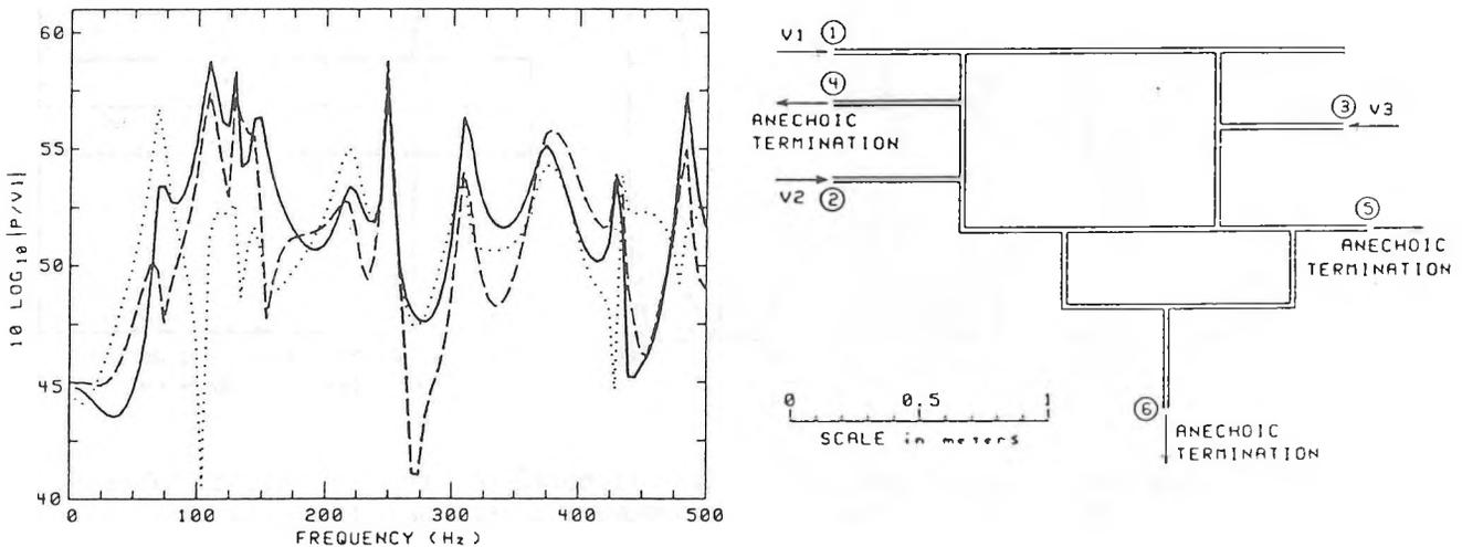
Figure 1. Piping network transfer impedance wrt Station 1
