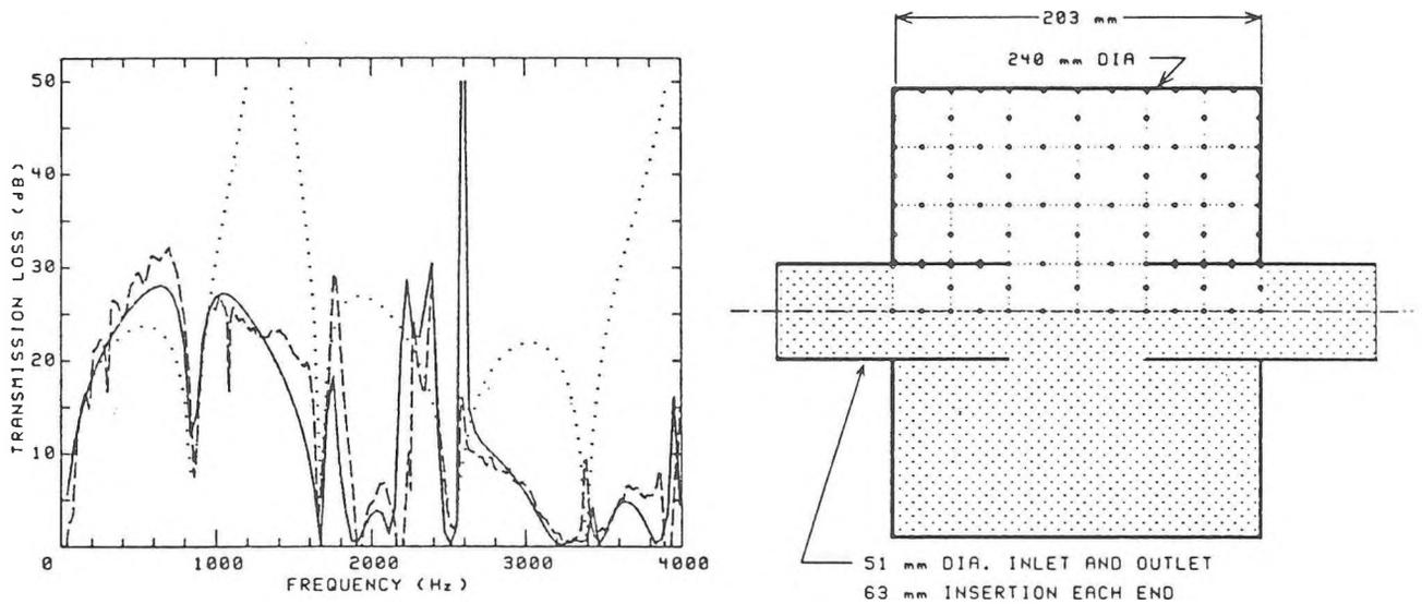
Figure 2. Axisymmetric expansion chamber with insertion tubes
