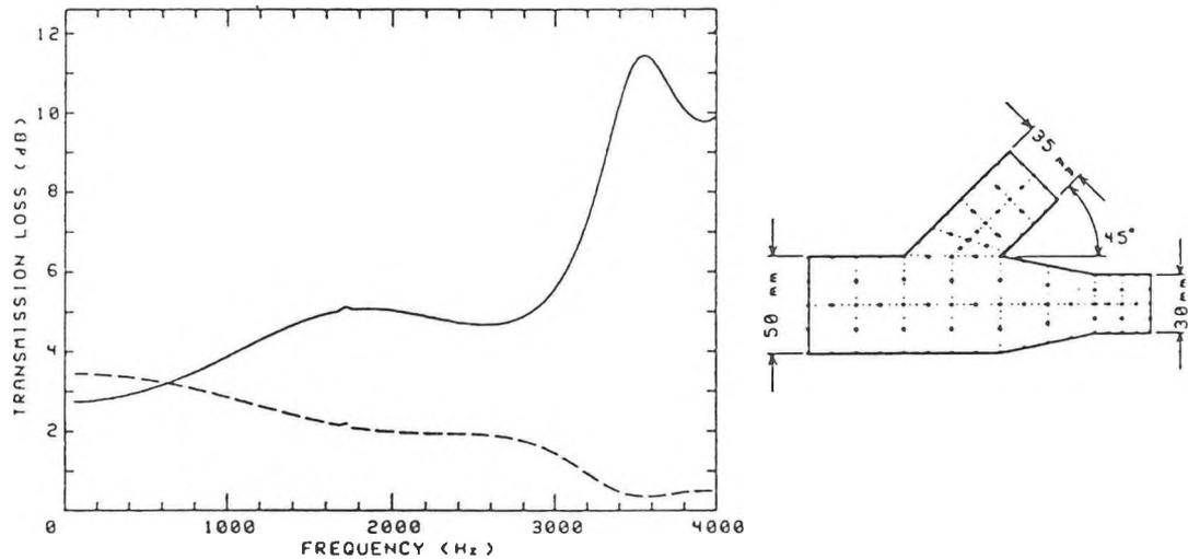
Figure 5. Rectangular duct with 45 degree branch
