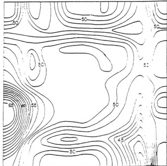
Figure 14. Transmitted Intensity at 1600 Hz after introduction of a fault. 1.14 m x 1.14 m panel
