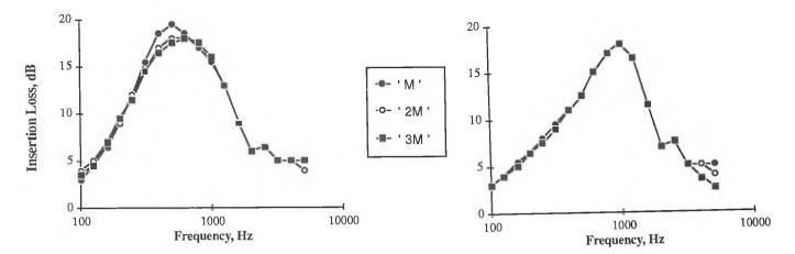
Figure 3. Insertion Loss of Splitter Silencers : M = 0.6 m, d / h =1 ; a) R = 8000 MKS Rayls / m, b) R = 20000 MKS Rayls / m
