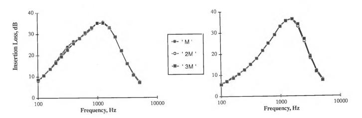
Figure 5. Insertion Loss of Splitter Silencers : M = 0.6 m, d / h =3; a) R = 8000 MKS Rayls / m, b) R = 20000 MKS Rayls / m
