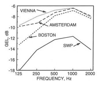
Figure 7. Comparison of hall-average GEL values versus octave band frequency.
