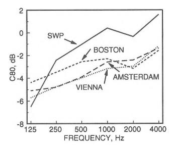
Figure 4. Comparison of hall-average C80 values versus octave band frequency.
