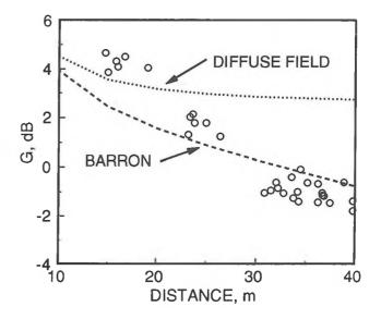
Figure 11. Comparison of measured 1 kHz G values with predictions of diffuse field theory and Barron's revised theory for SWP.
