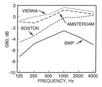
Figure 6. Comparison of hall-average G80 values versus octave band frequency.
