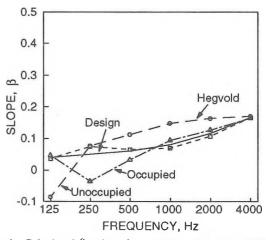
Figure 6. Calculated  $\beta$  values for upholstered theatre chairs with edges screened for occupied and unoccupied type E chairs. Also shown is a design curve approximating the calculated values and Hegvold's simple model audience results.
