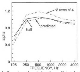
Figure 3. Comparison of sound absorption coefficients for type A chairs, measured in the hall and estimated from reverberation chamber tests for two rows of four chairs (P/A = 2.0) and for a hall sized sample (P/A = 0.8).
