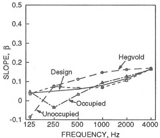
Figure 6. Calculated  $\beta$  values for upholstered theatre chairs with edges screened for occupied and unoccupied type E chairs. Also shown is a design curve approximating the calculated values and Hegvold's simple model audience results.
