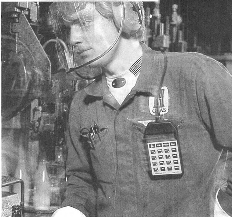
The Type 4436 dose meter can be used as a Type 2 integrating sound level meter.
