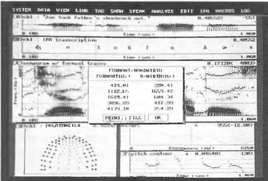
Multiple windows of analysis including speech waveform, phonetic transcription (time-linked to waveform), spectrogram with formant trace, LPC slice, pitch contour and linguapalatal contact in lower left is linked to cursor in spectrogram. Numerical window shows formants' center frequencies and bandwidths.
