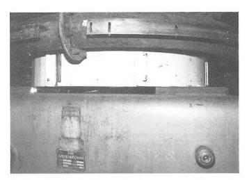
Photo 1. Acoustic Shroud around Coupling
