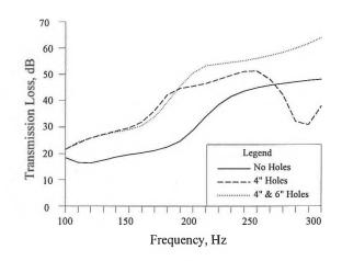
Figure 1: Predicted Transmission Loss of Various Wall Constructions
