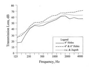
Figure 2: Field Transmission Loss Test Results for Various Wall Constructions
