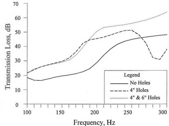
Figure 1: Predicted Transmission Loss of Various Wall Constructions
