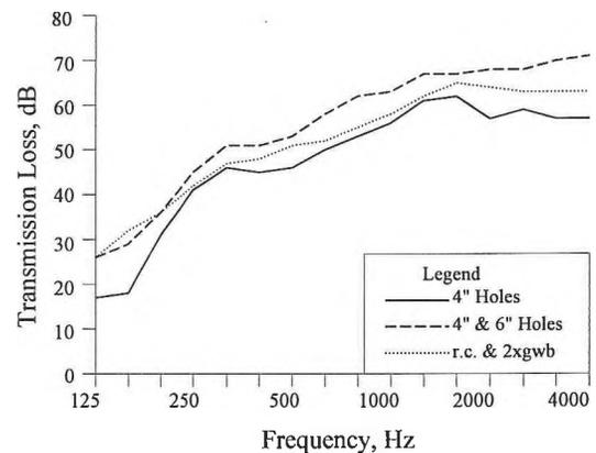
Figure 2: Field Transmission Loss Test Results for Various Wall Constructions
