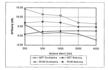
Figure 1 Stage to Pit Balance (SPB) measured by O'Keefe.
