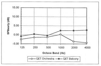
Figure 2 Stage to Pit Balance (SPB) extracted from Bradley's measurements.
