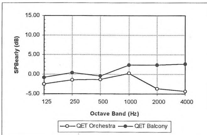
Figure 2 Stage to Pit Balance (SPB) extracted from Bradley's measurements.
