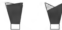
Figure 4 - classical shape of alternate teeth vs. high top bevel angle alternate teeth
