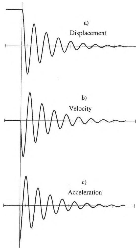
Fig. 1: Theoretical Vibration Decay Records for Pull-Release Test
