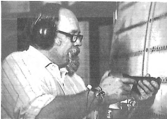
Photo 3. View of the riveter and the accelerometers
