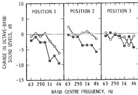
FIG. 12 Effect of baffles in inlet and outlet openings of enclosure at Site 1:
