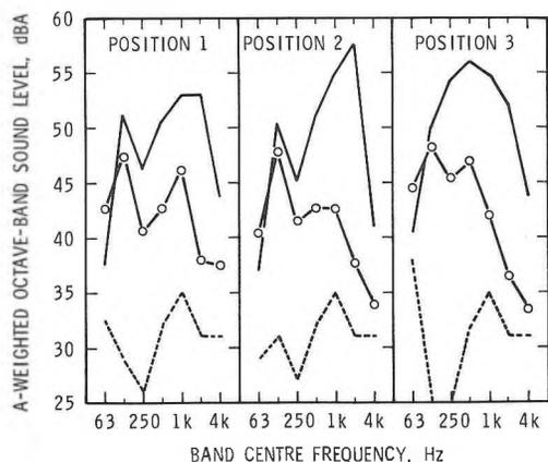
FIG. 7 Measured sound levels at Site 1:
