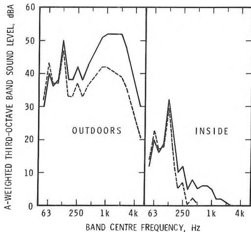
FIG. 13 Combined effect of enclosure and transmission through exterior wall: (—) sound levels without enclosure, (---) sound enclosure added. Outdoor level changes from 60 to 52 dBA. Indoor level changes from 33 to 31 dBA
