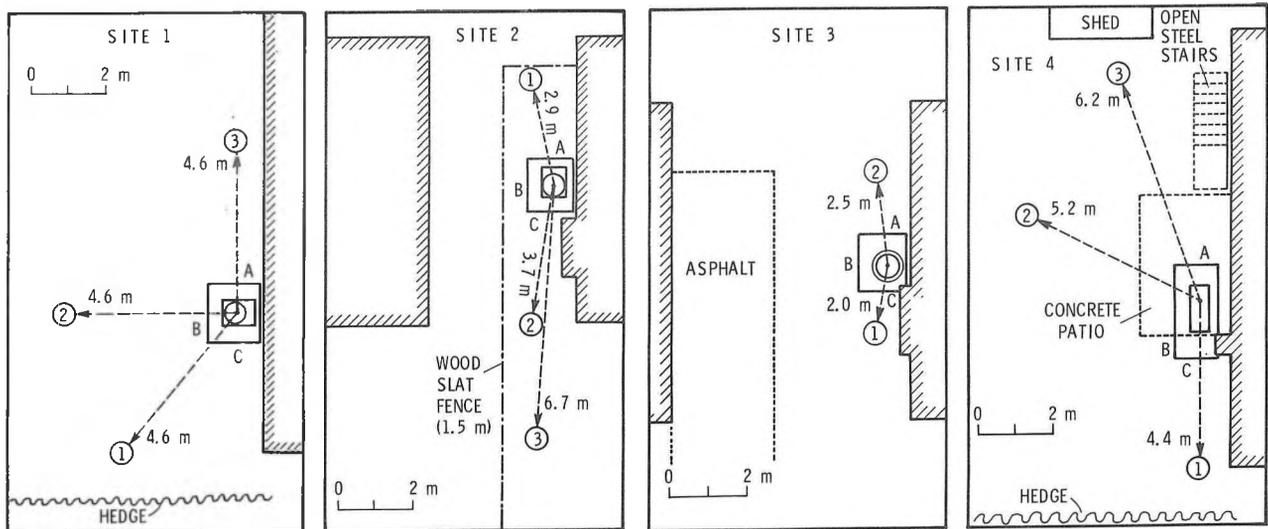
FIG. 6(a) Four test sites showing measurement positions (circled numbers) and site details.
