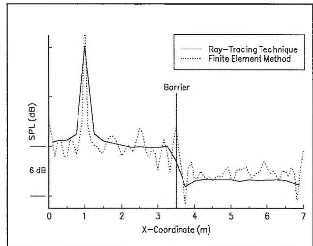
Figure 5 - Sound Levels due to Presence of Barrier
