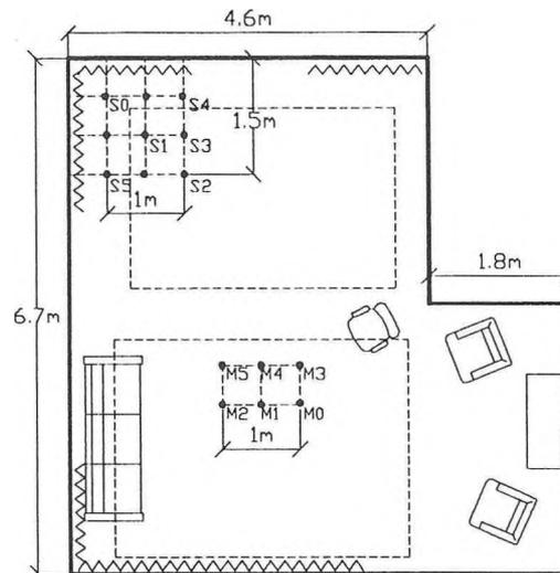
Figure 1. Listening room layout showing source positions S0 to S5 and measurement positions M0 to M5.
