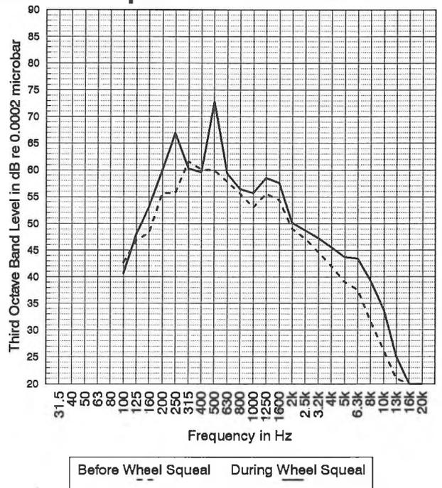
Fig 2: Spectral Comparison of Streetcar Before & During Wheel Squeal
