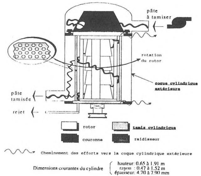
fig. 1 description of a pressure pulp screen
