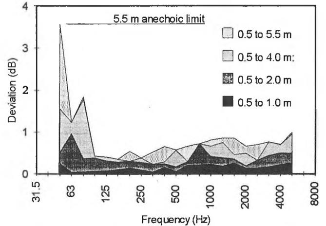
Figure 1: Measured maximum deviations from inverse square law for four source-receiver separation distances.
