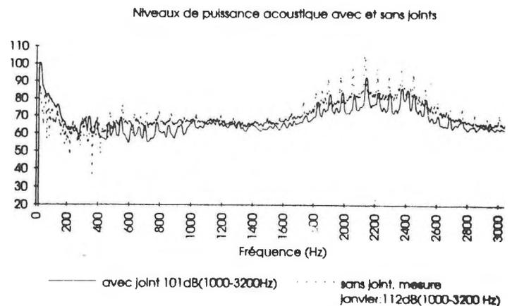
fig. 3: Effects on the global noise of a machinical isolation between the basket and the rest of the machine
