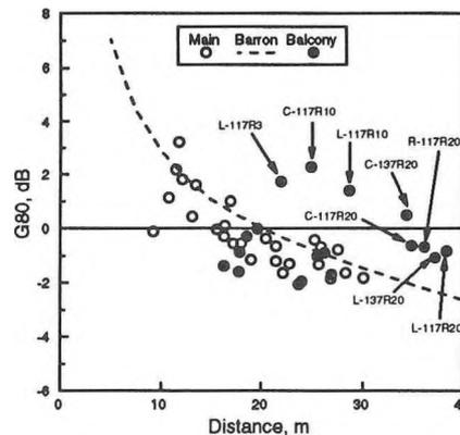
Figure 5. G80 values versus distance at 1000 Hz.
