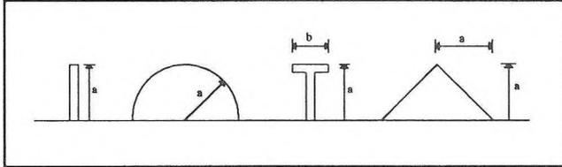
Figure 5 - Barrier Shapes with Dimension  $a=3\text{m}$ ,  $b=2\text{m}$
