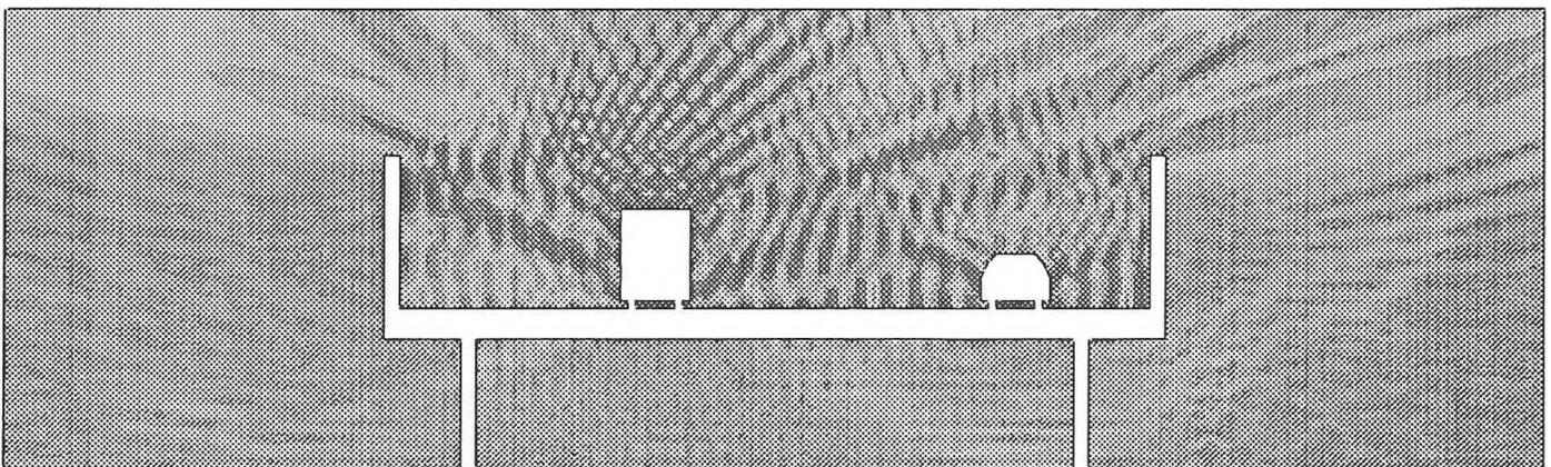
Figure 7 - Sound Pressure Contours for Raised Highway with Barriers
