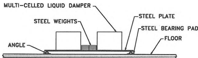
Figure 1. Prototype Damper
