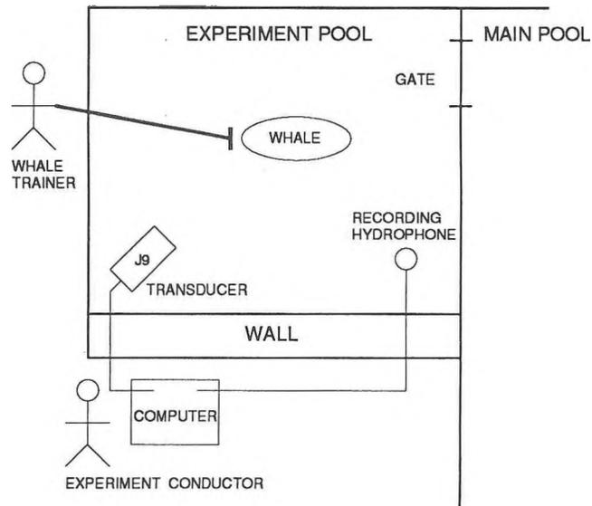
Figure 2: Experiment Set-up
