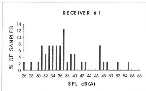
Figure 2 Distribution of the total Sound Pressure Level from two sources (320 and 440 Hz) of an industrial plant.
