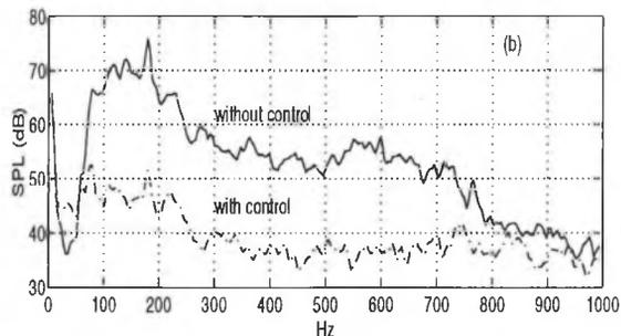
Fig. 3. (a) Spectrum of noise above headset; and (b) Active noise reduction performance.
