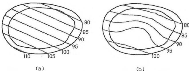
FIG. 4 Contours for the out-of-plane component of footplate displacement for (a) normal middle-ear model and (b) MFA model. All displacements are in nanometres (nm).
