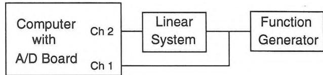
Figure 1. Diagram of equipment used in pure-tone tests.
