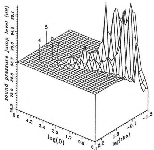
fig 4: Sound pressure jump level at 90 Hz as a function of  $\log(\rho_s)$  and  $\log(D)$  where  $\rho_s$  is the mass per unit area and  $D$  is the flexural rigidity. #1-#2 : 5 mm. and 1 cm. of aluminium, #3-#4 : 5 mm. and 1 cm. of steel, #5 : typical sandwich panel.
