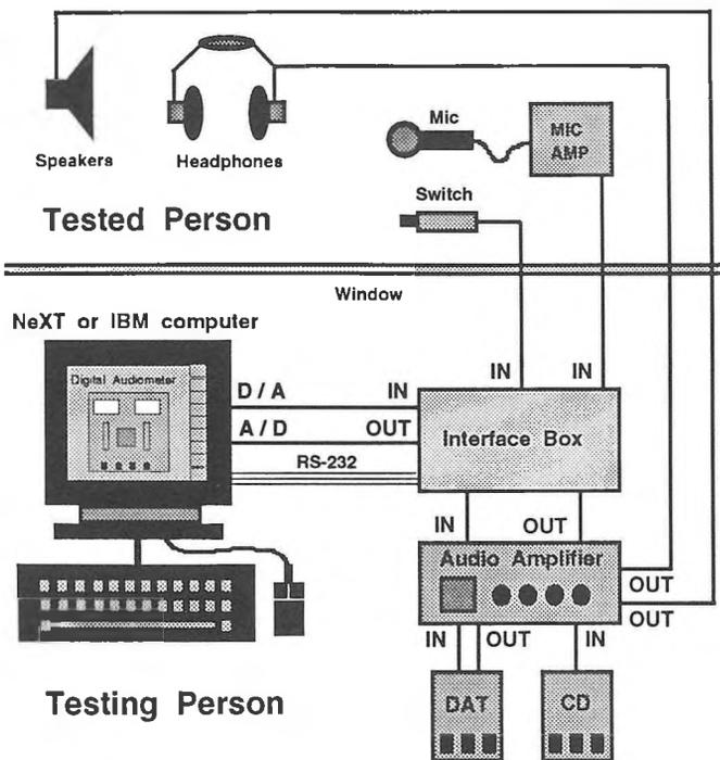
Fig. 1. Schematic Diagram of the Digital Audio Laboratory
