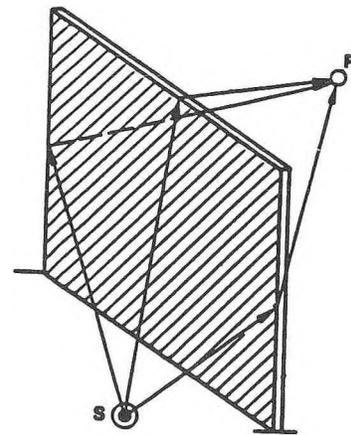
Figure 2. Different sound propagation paths at a screen
