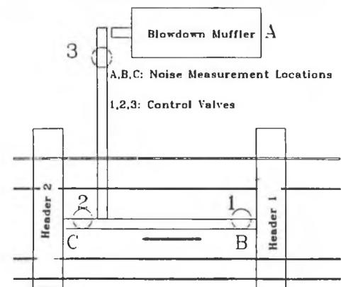
Figure 1. Lay Out of a Transfer Station
