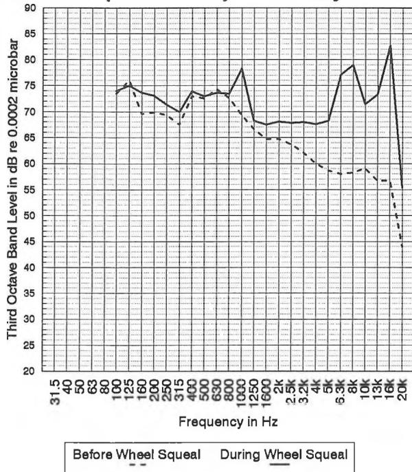
Fig 1: Spectral Comparison of Subway Before & During Wheel Squeal
