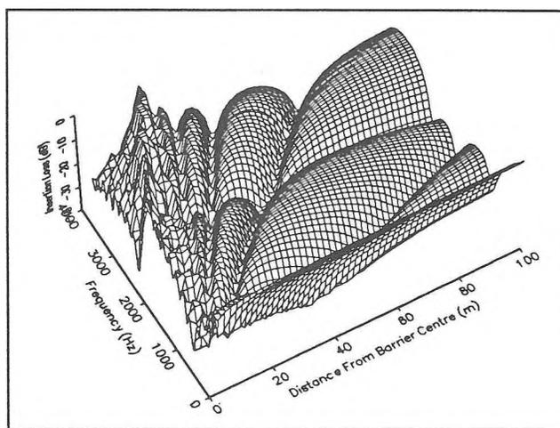
Figure 3 - Thin Barrier Insertion Loss - broadband
