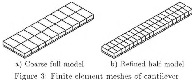
Figure 3: Finite element meshes of cantilever
