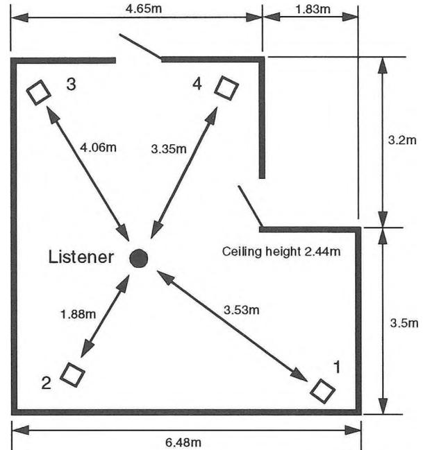
Figure 1. Layout of listening room illustrating listener and numbered loudspeaker positions.
