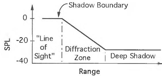
Fig. 1 Upward Refraction
