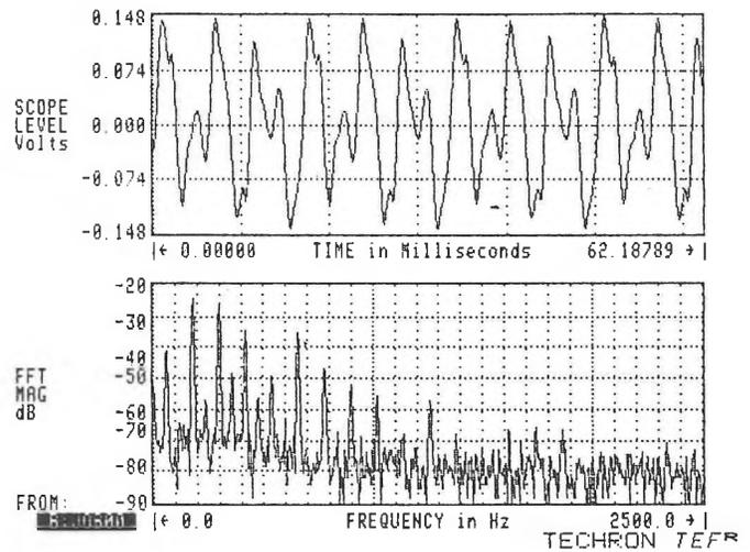
Fig 2. AC Line related noise spectrum.
