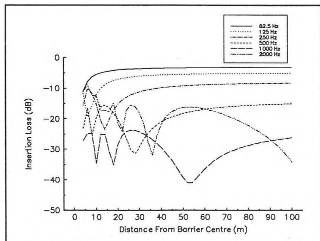
Figure 2 - Thin Barrier Insertion Loss - octave center freq's
