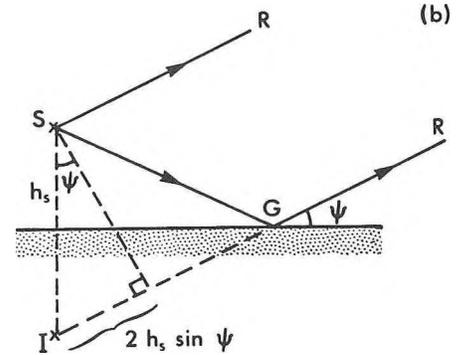
Figure 1. Sound propagation paths downwind
