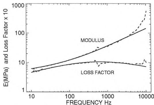
Figure 2: C-1002 properties (— Fitted, - - - Measured)
