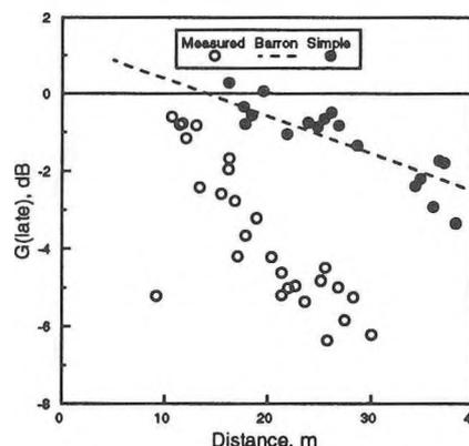
Figure 6. G(late) values versus distance at 1000 Hz.
