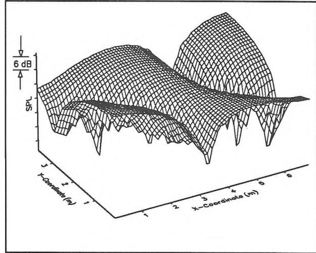
Figure 2- SPL at 50 Hz - 10% Absorption
