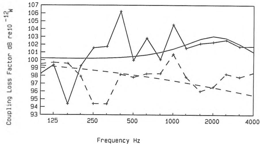
Figure 1. Measured and predicted coupling loss factors for transmission from a concrete column to a plate/beam.— predicted (symmetric); +— measured (symmetric); -- predicted (asymmetric); -x- measured (asymmetric).
