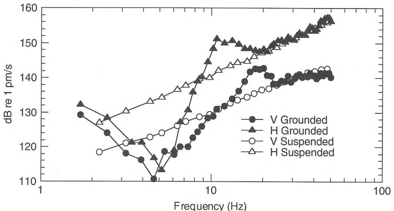
Fig. 2. Results of a coupling test. The values shown are the vertical and horizontal amplitude response of the OBS to an integral vibrator in two conditions: suspended in water, and grounded on a typical sea floor.
