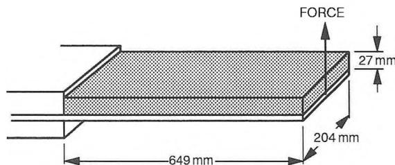
Figure 1: Steel cantilever with 27 mm thick damping layer
