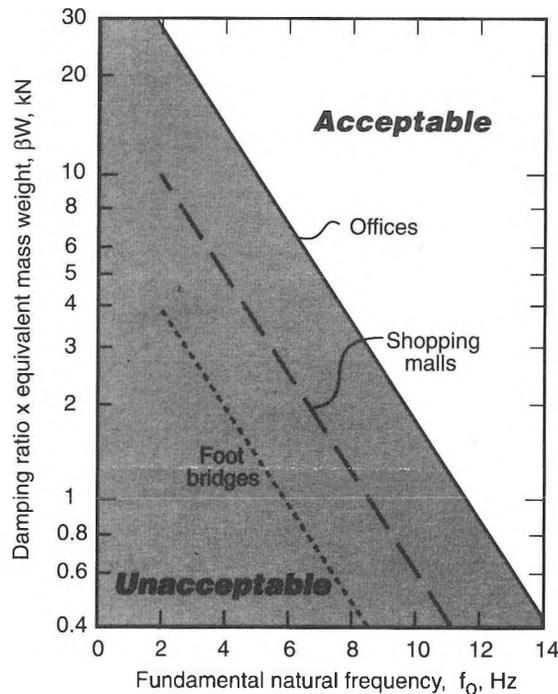
Figure 1. New Design Criterion for Walking Vibrations
