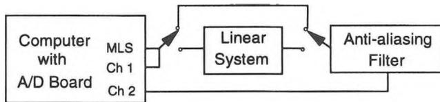
Figure 2. Diagram of equipment used in m-sequence tests.
