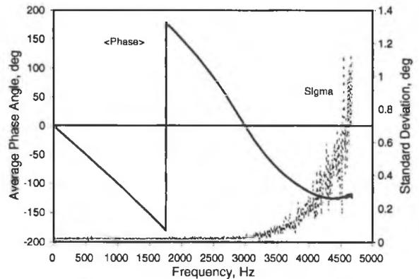
Figure 3. Average and standard deviation of the phase response of a 3 kHz low-pass filter from 10 measurements.
