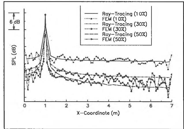
Figure 4 - Response in Room at Different Absorption Levels
