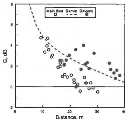
Figure 4. G values versus distance at 1000 Hz.
