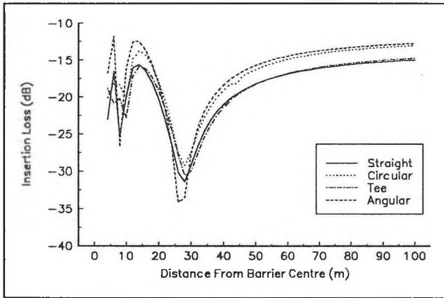
Figure 6 - Insertion Losses of Various Barrier Shapes
