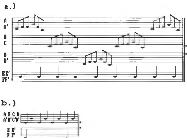
Fig. 2 Musical scores illustrating process of generating the "moving source" (a) and the "steady source" signals (crossing points denoted as in fig. 1).
