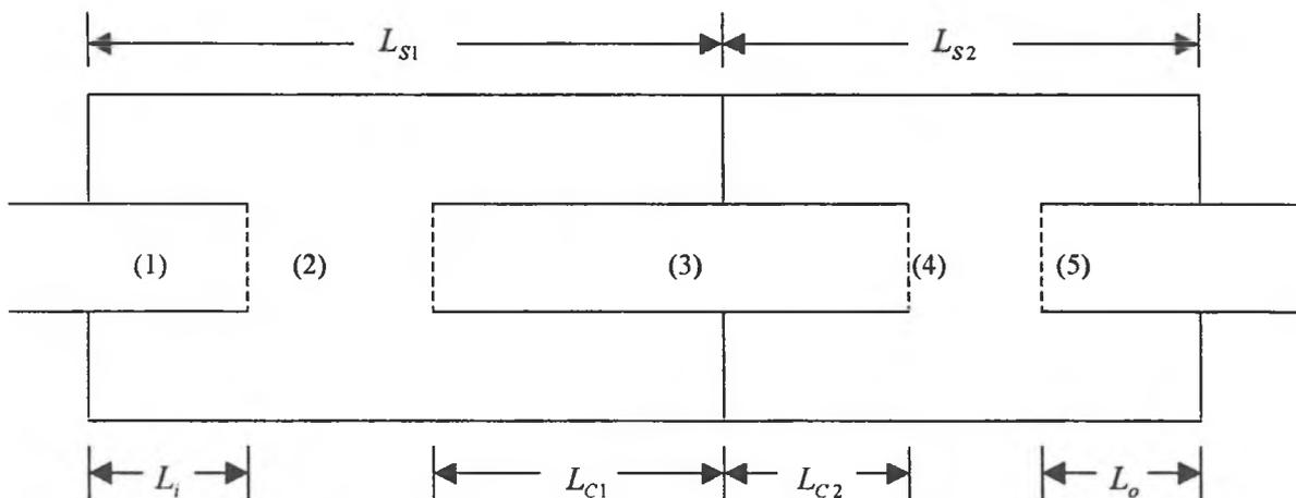
Figure 1. Double expansion chamber silencer with inter-connecting tube.
