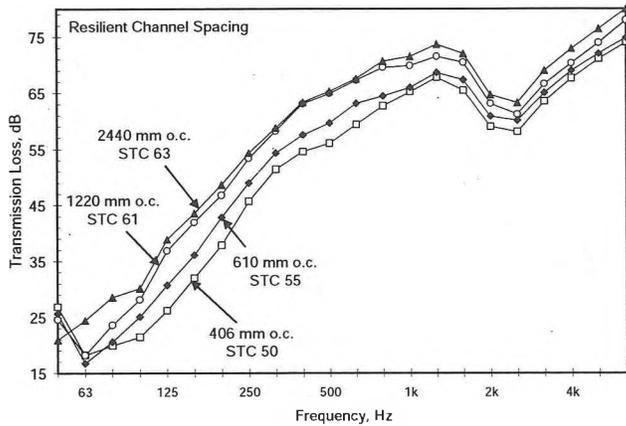
Figure 4: Changing resilient channel spacing in constructions G16\_OS B13\_WS89(406)\_GFB89\_RC13(xxx)\_2G16.
