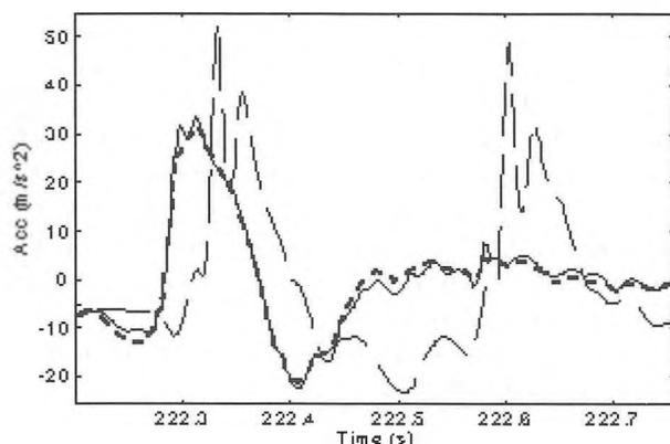
**Figure 1.** Acceleration ( $\text{m}\times\text{s}^{-2}$ ) measured at the seat (solid) and lumbar spine (long dash) and Wk frequency weighted acceleration (short bold dash) for a +4 g, 5 Hz z-axis mechanical shock.
