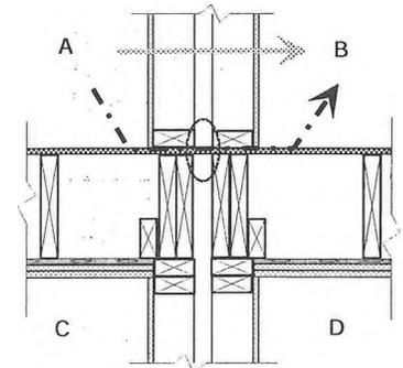
The floors had wood 2x10 joists, with joists parallel to the party wall (as in Fig 2), or perpendicular to the wall with each set of joists supported on one row of studs. Changing joist orientation had little effect on FSTC for this wall/floor combination. The sub-floor membrane was 5/8" oriented strand board (OSB) for most specimens. Substituting plywood caused negligible change.
