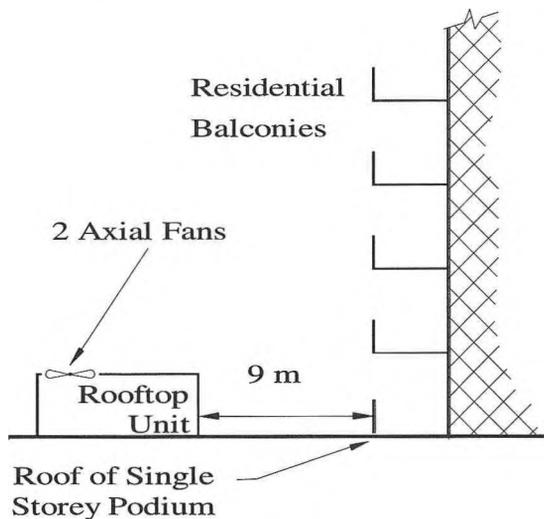
Figure 1: Sketch of Installation
