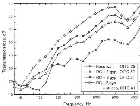
Figure 4. Effects of adding resilient channels (RC).
