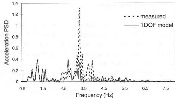
**Fig. 3 : Comparison of acceleration PSD of seat model with single-DOF occupant model with mean measured response**
