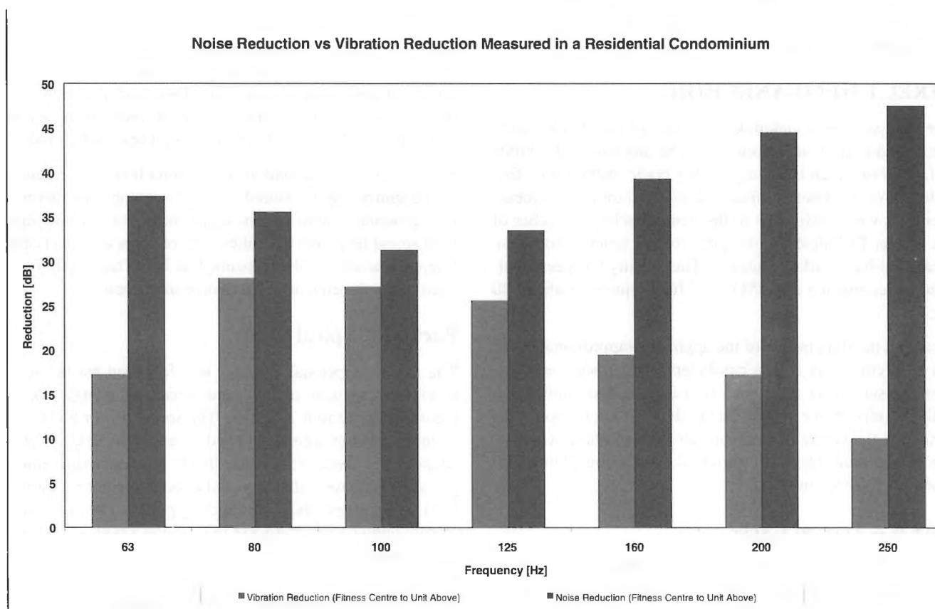
**Figure 1: Noise reduction compared to vibration reduction measured between a fitness centre and the unit above. Typical sources of impacts in the fitness centre were simulated, such as the skipping of rope, the dropping of weights, and treadmill activity. Those activities did not provide sufficient signal to noise ratios in frequency bands outside of the 63 to 250 Hz range, and were excluded from the results.**
