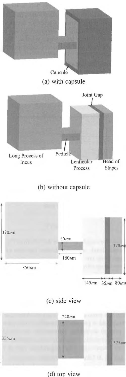
Figure 2: Shape and dimensions of the finite-element model
