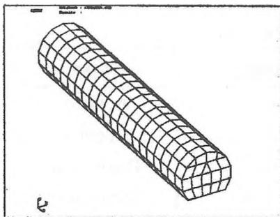
Figure 2. Boundary element model of a simplified aircabin
