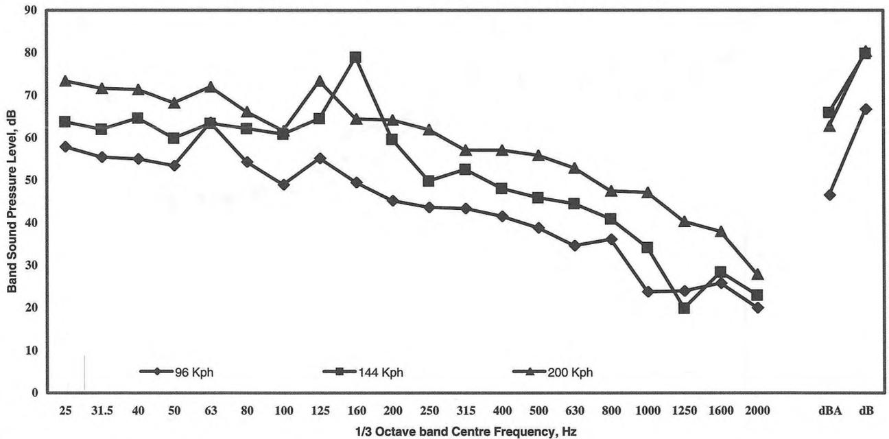
Figure 4. Control Room Noise Levels with weights on the Support Plate.
