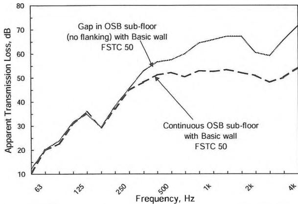
**Figure 3:** Effect of flanking transmission via the continuous OSB sub-floor in the case with the basic party wall.
