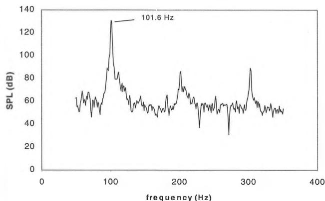
**Figure 2b: Measured Peak SPL (101.6 Hz) for a Vertical Traverse, Fan speed = 450 rpm, (0,3) mode, settling chamber height = 5080 mm**
