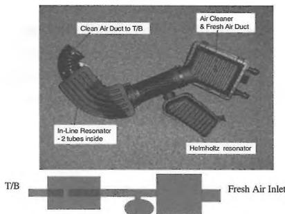
Figure 3. Daimler Chrysler LH 3.5L induction system.
