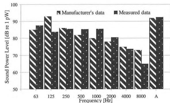
Figure 2: Sound Power Levels of Existing Rooftop Unit
