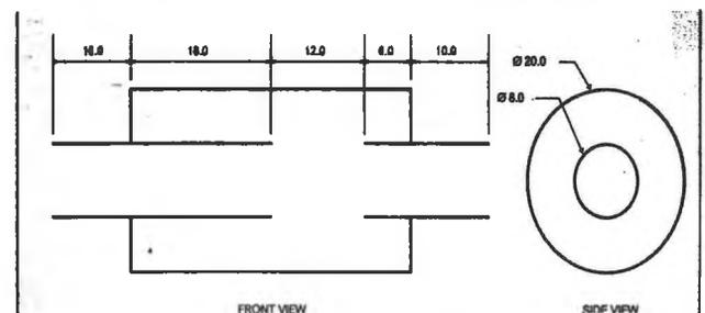
Figure 1. Dimension diagram (in cm) of expansion chamber.
