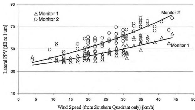
Figure 3a: PPV at Monitor 1 vs Monitor 2 - Lateral
