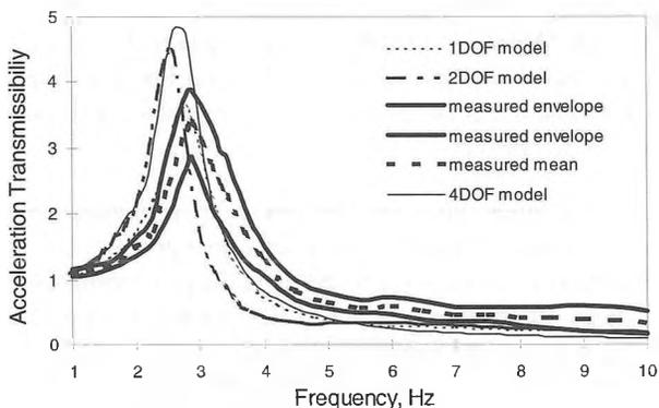
**Fig. 2 : Comparison of computed and measured acceleration transmissibility of the seat-occupant system.**
