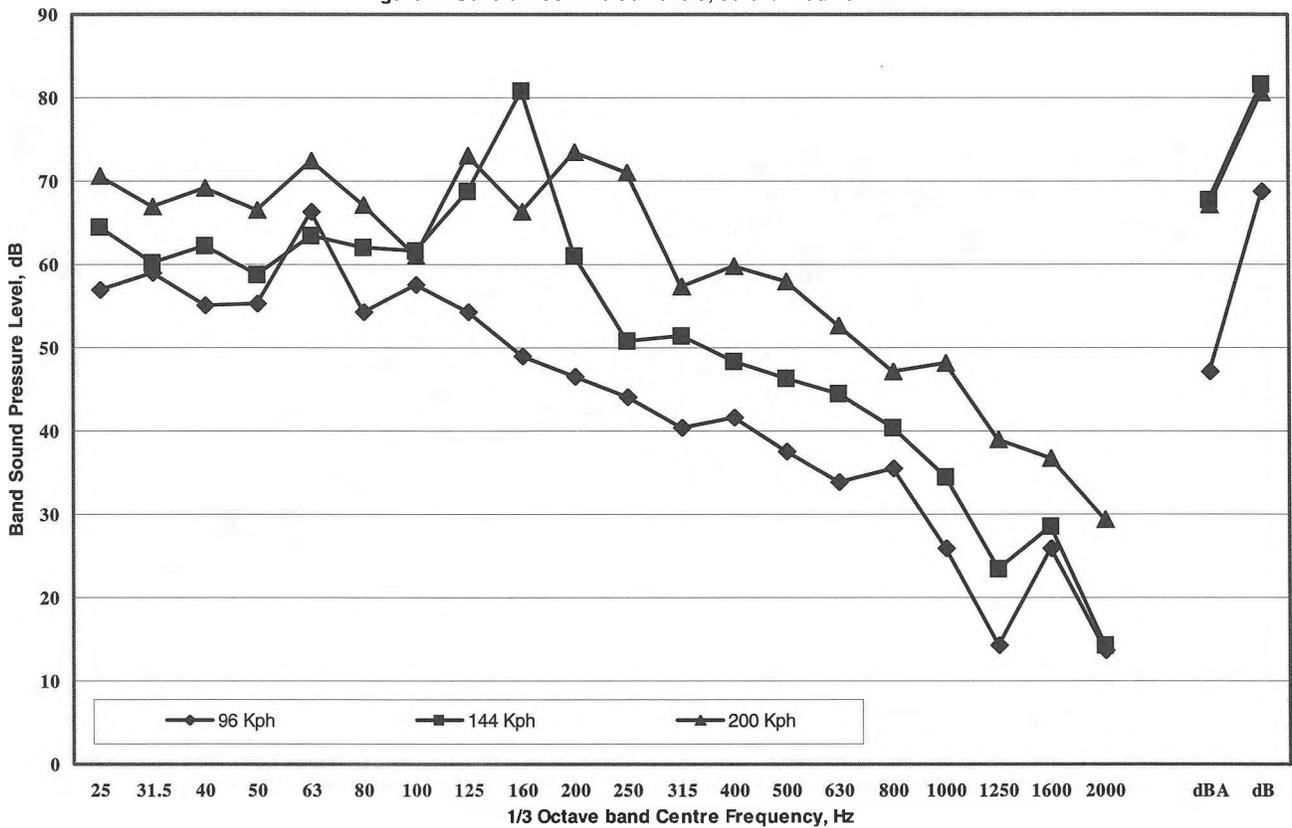
Figure 3. Control Room Noise Levels, with Fibreglas in the Settling Chamber.
