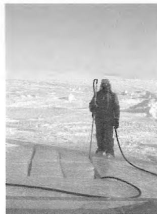
Fig. 3. A hot water drill is used to cut blocks of ice. The cut area will be large enough to accommodate the Phantom: a large, remotely-operated vehicle used to deploy our gear underneath the ice.
