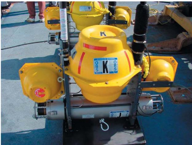
Figure 2. An OBH ready for deployment from the research ship.
