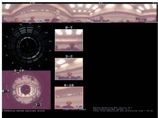
Fig. 2. Panocam. The raw video image appears in the lower left. The initial corrected panoramic image appears at the top. The real-time audio search response shows an active talker near 12:00 in the left centre frame and three virtual images are shown in the centre frame. The audio and corresponding virtual video (lower image, "6-10") is selected for output.
