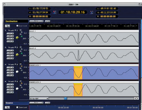
Figure 3. Audio waveform with clipping (top) and corrected (bottom). Total length of audio shown is 9.6 ms.
