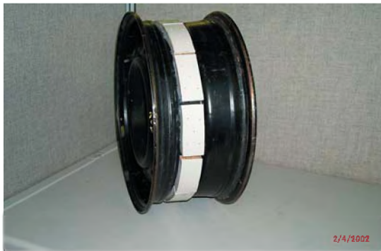
Figure 7. Resonators are wrapped around the dip of the base
