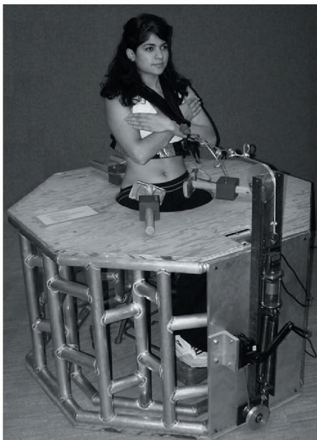
Figure 1. Apparatus used to fix the pelvis and allow isometric trunk contraction such as extension (shown) and lateral flexion.
