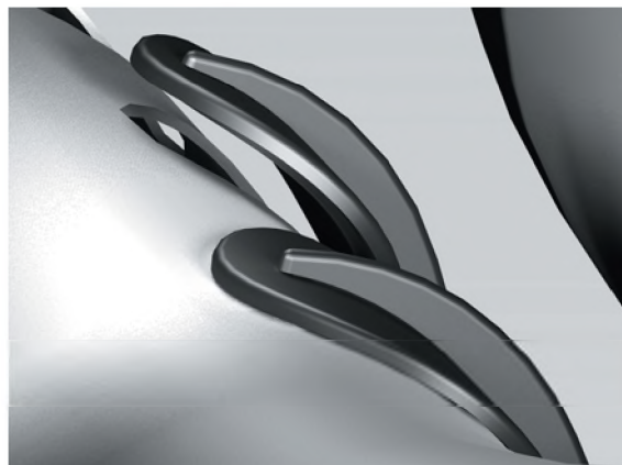
Fig. 2. Experimental tonehole design without chimney.
