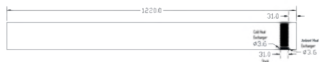
Fig. 1. Sketch of the thermoacoustic refrigerator with air, all dimensions are in millimeters
