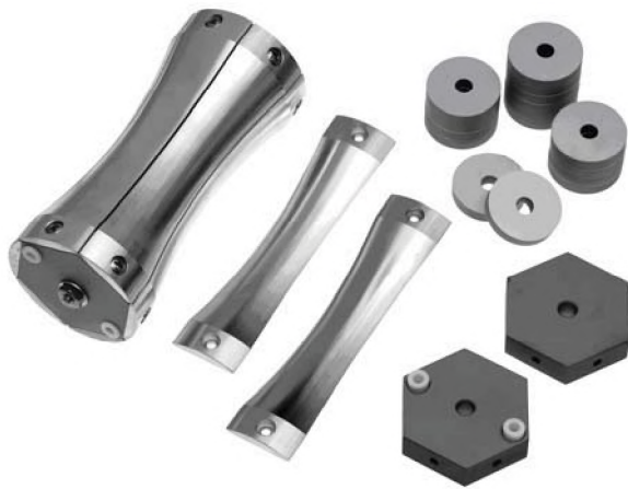
Figure 1: Barrel-stave flextensional transducer components clockwise from upper right: sixteen piezoceramic washers, two ceramic glass insulators, two hexagonal endplates, six concave aluminum staves (the two shown separately are 12.7 cm long), and a stress rod located along the axis of the transducer.
