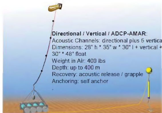
Figure 3 : Vertical array/directional hydrophone data acquisition system.
