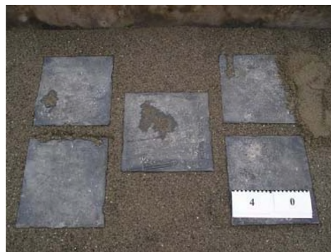
Fig. 4: Structural Isolation Pads, immersed in Compacted Sand
