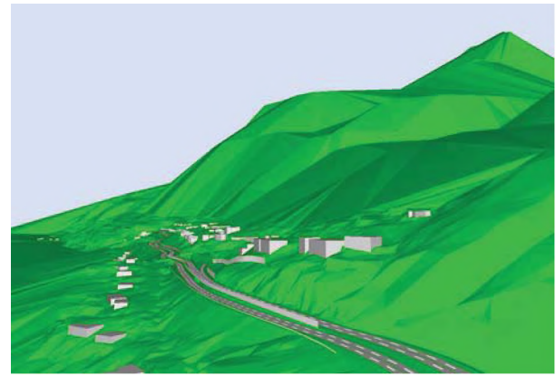
Figure 1.1: View of Sea-to-Sky Highway through Lions Bay from Vancouver End towards Whistler, showing Proposed Four Lane Configuration with 750 m Split Grade Section.
