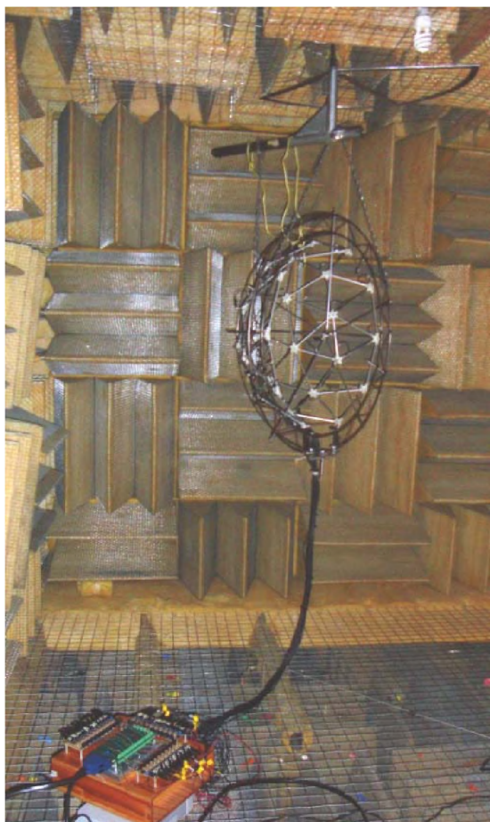
Figure 1. Antenna and DAQ system in anechoic chamber.
