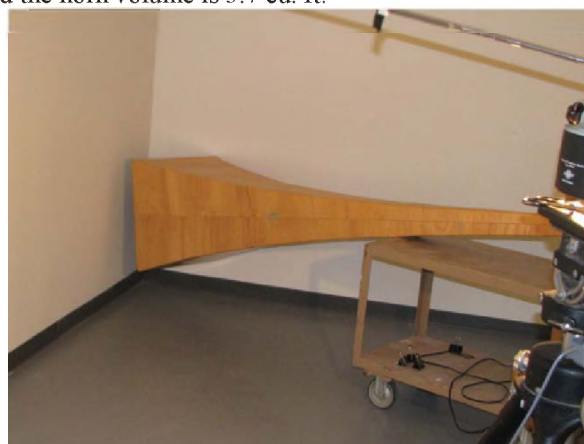
Figure 1. The Hyperbolic horn at a triple corner (The microphone boom is in the background).
