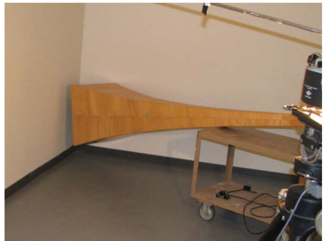
Figure 1. The Hyperbolic horn at a triple corner (The microphone boom is in the background).
