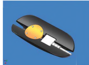
Figure 1. Adaptor with triaxial accelerometer.
