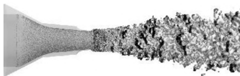
Figure 1. SMC nozzle: 0.9 jet Q-criterion isosurface.
