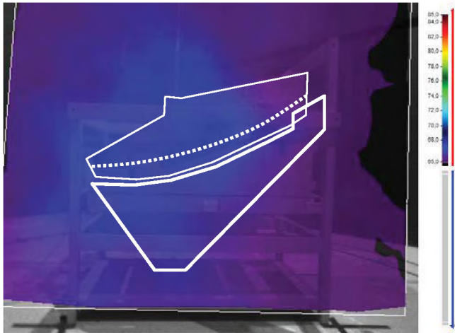
Figure 4. Slotted screen plate and current hopper - side 205 to 235 Hz global level L_1 = 72 dB
