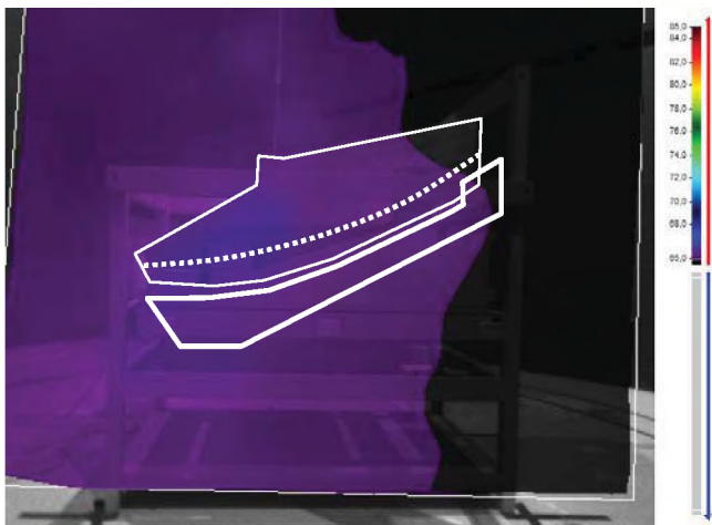
Figure 5. Slotted screen plate and proposed hopper – side 205 to 235 Hz global level L_1 = 67 dB
