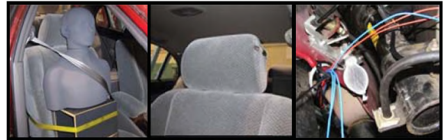
Figure 9: (Left) passenger's seat with binaural head; (Middle) driver's seat with conventional microphone; (Right) microphone next to the front wheel
