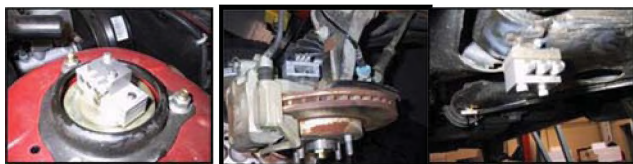
Figure 8: (Left) top of the McPherson strut; (Center) bracket next to wheel hub; (Right) lower A-arm
