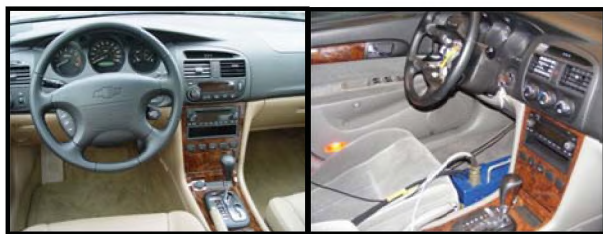
Figure 7: (Left) original Epica's interior; (Right) modified interior-airbag removed
