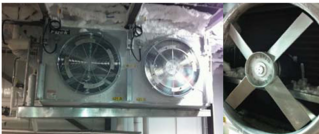
Figure 1. Left: example of flow control obstructions installation (upstream view). Right: rotor and its environment (strut, ice accretion, radiator...)
