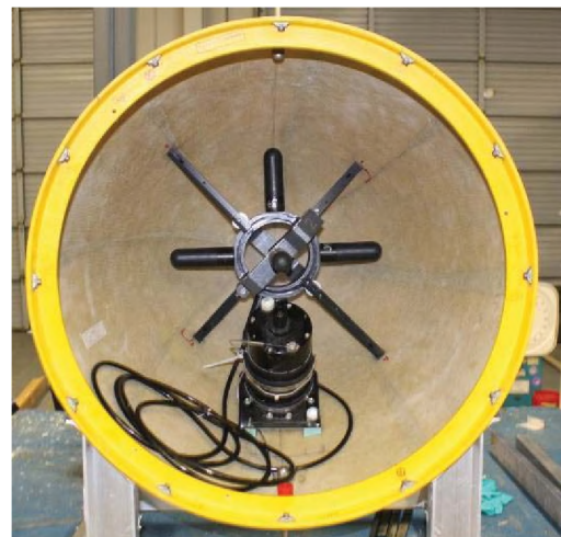
Figure 2. The LRAB array in the ISE Explorer nose cone.
