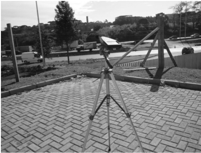
Figure 2. BK 2260 sound pressure level meter – Measurement point no. 3, facing the Green Line, Leq = 71.7 dB(A) (see Table 2).
