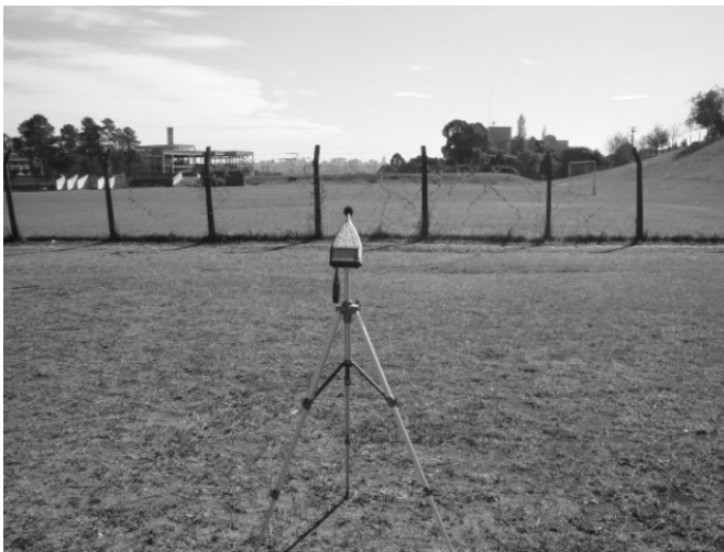
Figure 3. BK 2260 sound pressure level meter – Measurement point no. 20, green area of the campus, Leq = 51.4 dB(A) (see Table 2).
